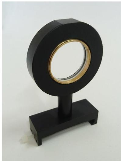
**Fig. 10. The large collimator lens of spectroscope.**
