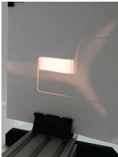
**Fig. 19. The sharp image of the bulb filament on the screen.**
