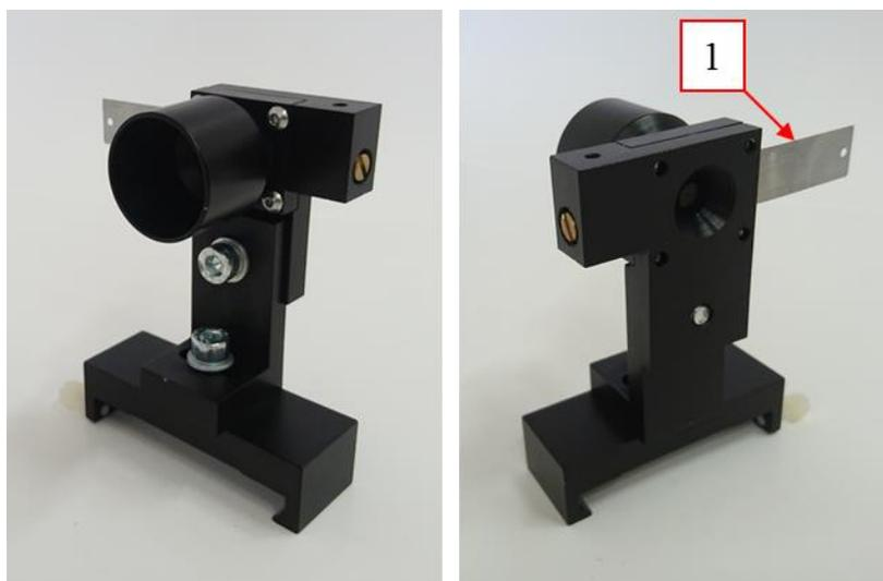
**Fig. 9. The entrance slit of spectroscope.
