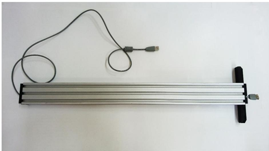
**Fig. 6. The optical rail.**
